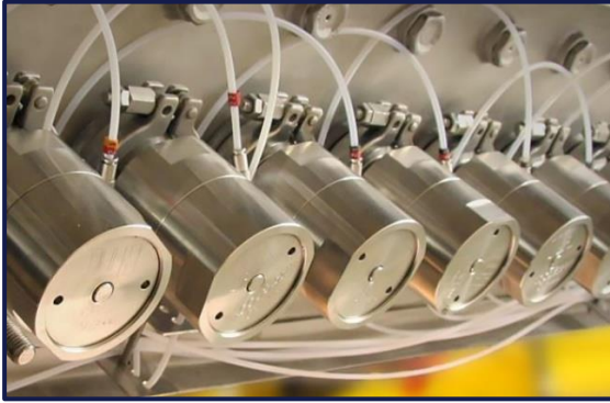
Img.2. Zone control valves
